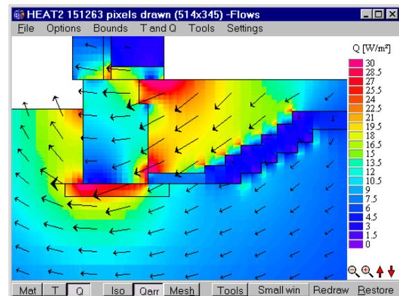
Slab on the ground. Top figure shows temperature field. Bottom figure shows heat flow intensity with large thermal bridge effects indicated by red color. Heat flow arrays are also shown.
