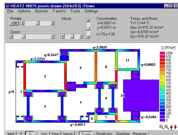
Window frame with 11 cavities. This steady-state problem with 10000 numerical nodes takes a few seconds to solve with a Pentium 3.
